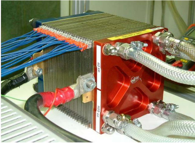
Fig. 7. Twenty-four-cell stack with non-machined bipolar plates under test.
